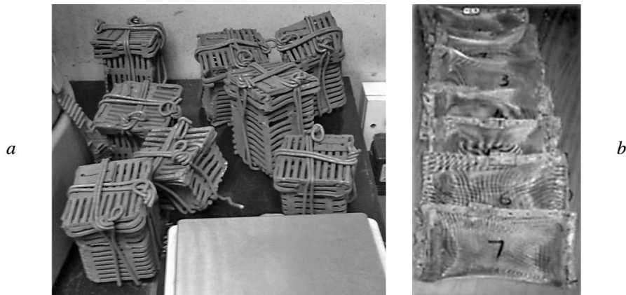
Fig. 3. Steel cages ( a ) and packets ( b ) for charging briquettes together with pellets into a Midrex reactor.
