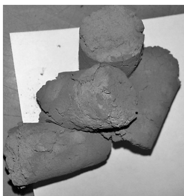
Fig. 5. Agglutination of 01-02 briquettes during solid-phase reduction.
