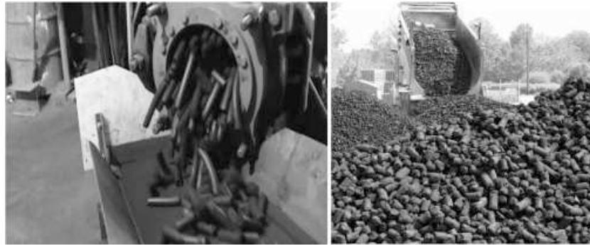
Fig. 9. Production of the BREX by Steele 75 Extruder (left) and discharge of the green BREX after 5–15 minutes at the storage area (right).
