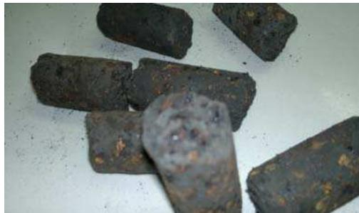
**Figure 8.** Brex made from HBI fines.
