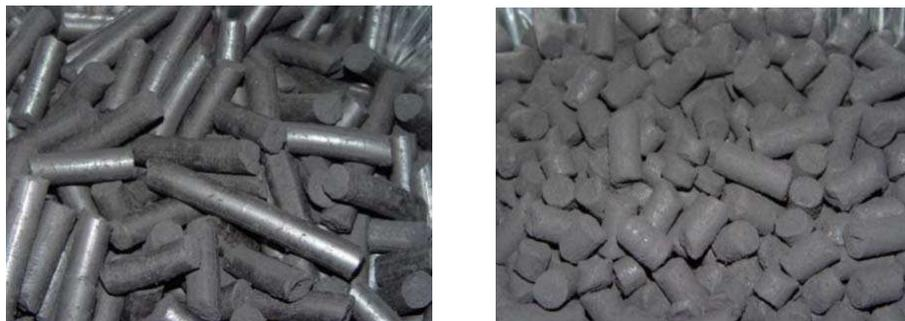
**Figure 7.** Coke breeze brex prior and after the tumble in rotating drum.
