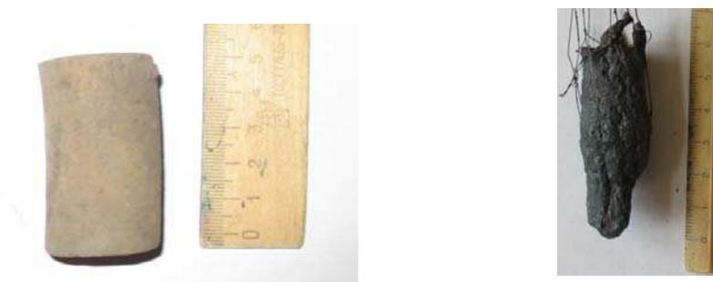
**Figure 6.** Sample #2-3 before and after thermal exposition at T= 1500°C.
