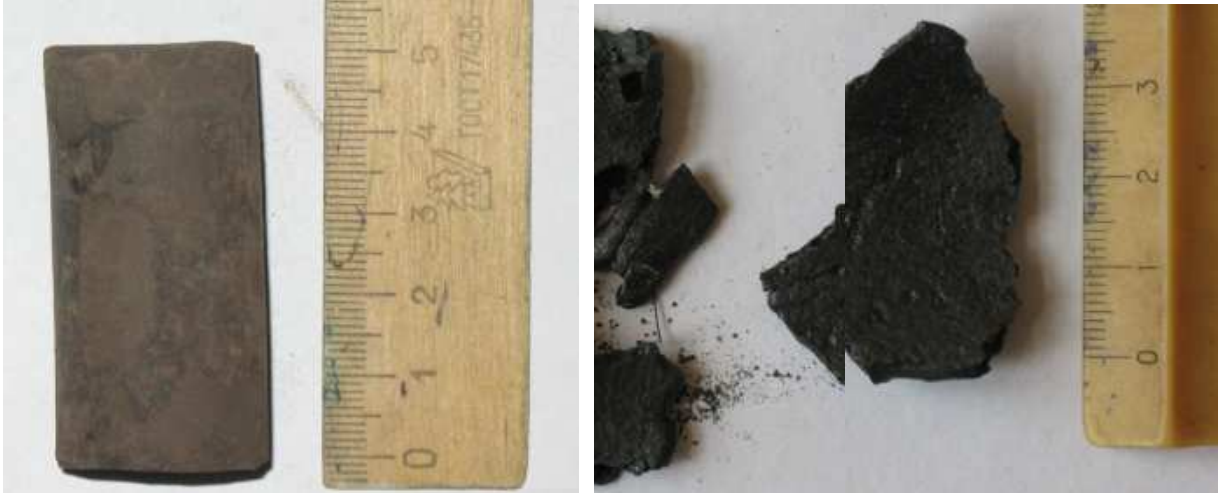
Fig. 7: Sample №1 before and after thermal shock at T = 1500^{\circ}\text{C} .
