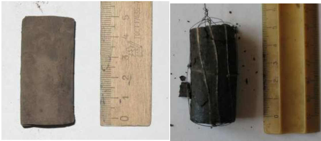
Fig 5: Sample №3 before and after thermal shock at t = 1200^{\circ}\text{C} .
