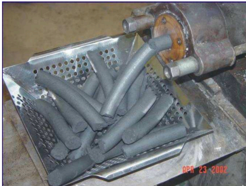
Figure 1: Laboratory Extrusion Testing
