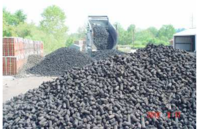
Figure 10: Dumping Green Brex within 2-20 min. after Extrusion
