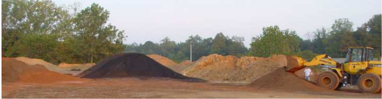
Figure 8: Blending Mn Ore and Furnace Dust On Site
