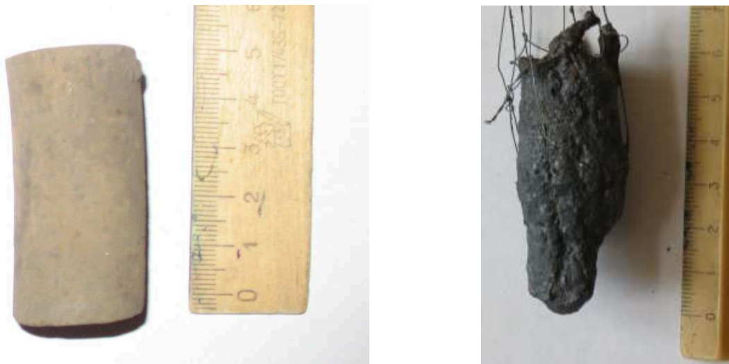
Fig. 6: Sample №2 before and after thermal shock at T = 1200^{\circ}\text{C} .
