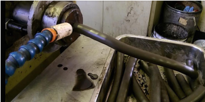
Fig. 25.40 Production of bentonite bonded chromium ore fines brex on a laboratory extruder
