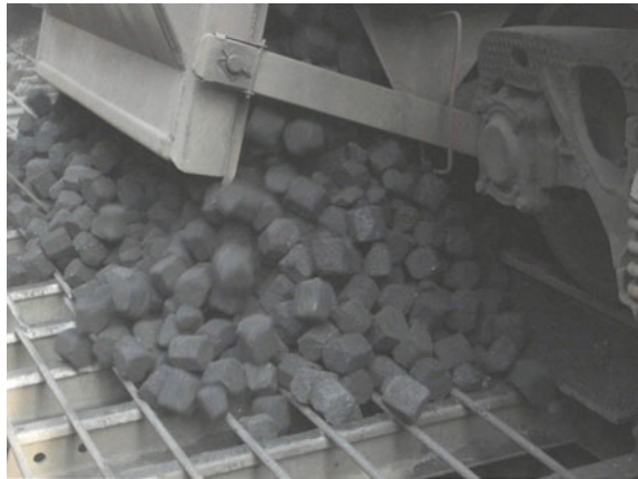
Fig. 25.15 Unloading of vibropressed briquettes from the car
