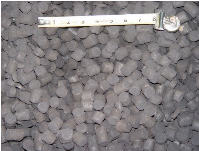
Fig. 25.48 Extruded brex for pilot testing of partial metallization of chromites in RHF
