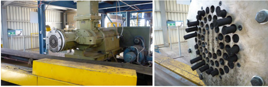
Fig. 6.2 The appearance of SVE extruder (J.C. Steele & Sons, Inc), and the brex coming out of the die
