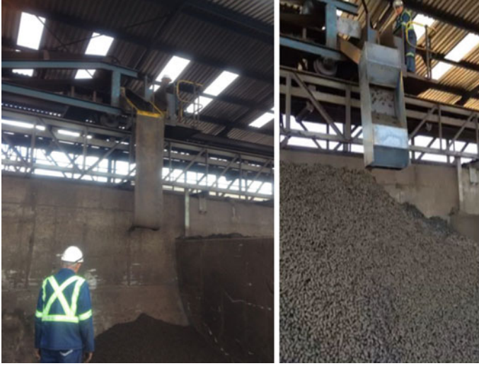
Fig. 2.33 Unloading of green bauxite in the bunker with a height of over 5 m
