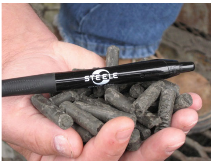
Fig. 6.4 TXI lightweight aggregates produced by SVE
