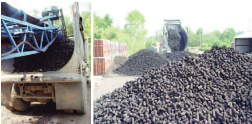
Fig. 2.32 Loading of freshly formed brex onto a dump truck and its subsequent unloading 5 min later
