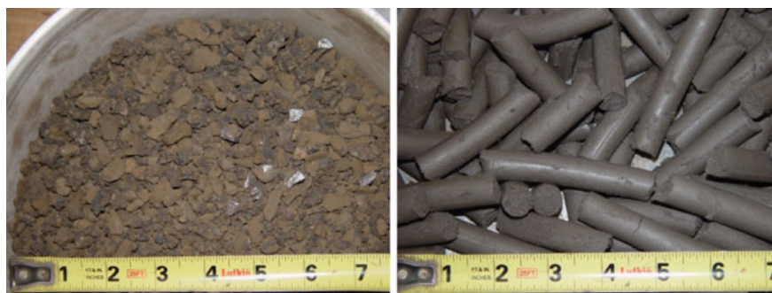
Fig. 4.20 Silicomanganese crushing fines (left) and brex based on Silicomanganese crushing fines (right)
