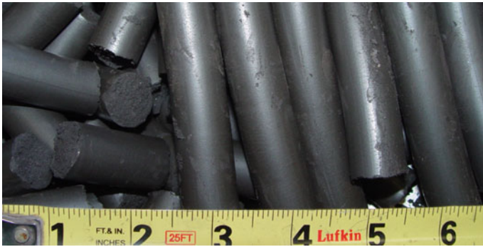
Fig. 4.27 Green brex made of chromium ore fines and aspiration dusts
