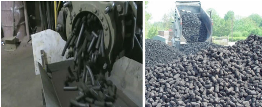
Fig. 4.16 Production of the brex by Steele 75 Extruder (left) and discharge of the green brex after 5–15 min at the storage area (right)
