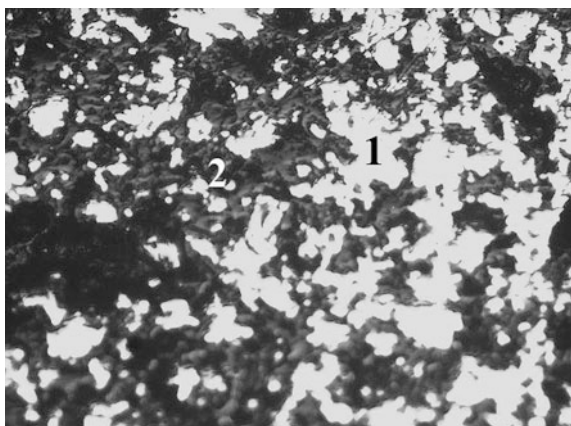
Fig. 5.11 Optical microscopy of the reduced lime-bonded brex (1—iron, 2—Melilite; magnification 200)
