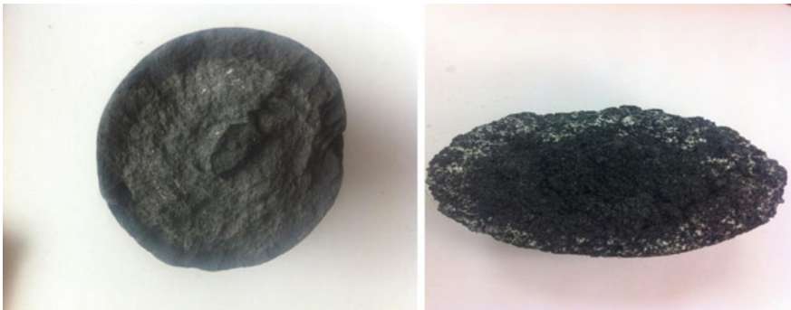
Fig. 2.28 Brex with a layer of fine fraction on the surface. Left: coal (surface layer) and fine fraction of construction materials. Right: coke brex with epoxy resin as binder
