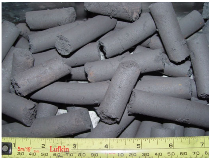
Fig. 4.24 Brex from FS 75 fines and aspiration dust
