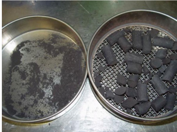
Fig. 2.40 Breaking of brex (after 48 h of preparation) after a five drops from a height of 2 m
