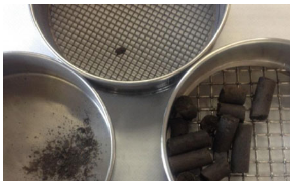
Fig. 2.39 Test results for a four-time drop from a height of 1.5 m of brex No. 2
