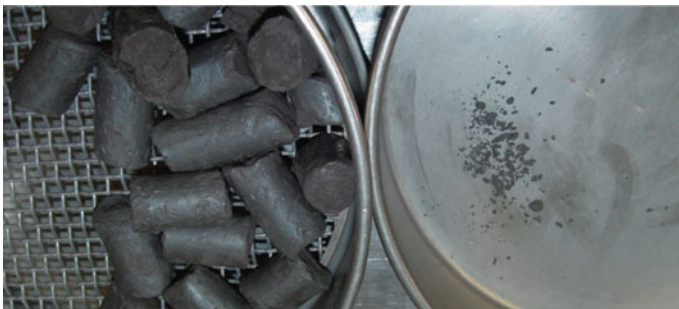
Fig. 4.28 Results of the drop test of brex made of chromium ore fines and aspiration dusts
