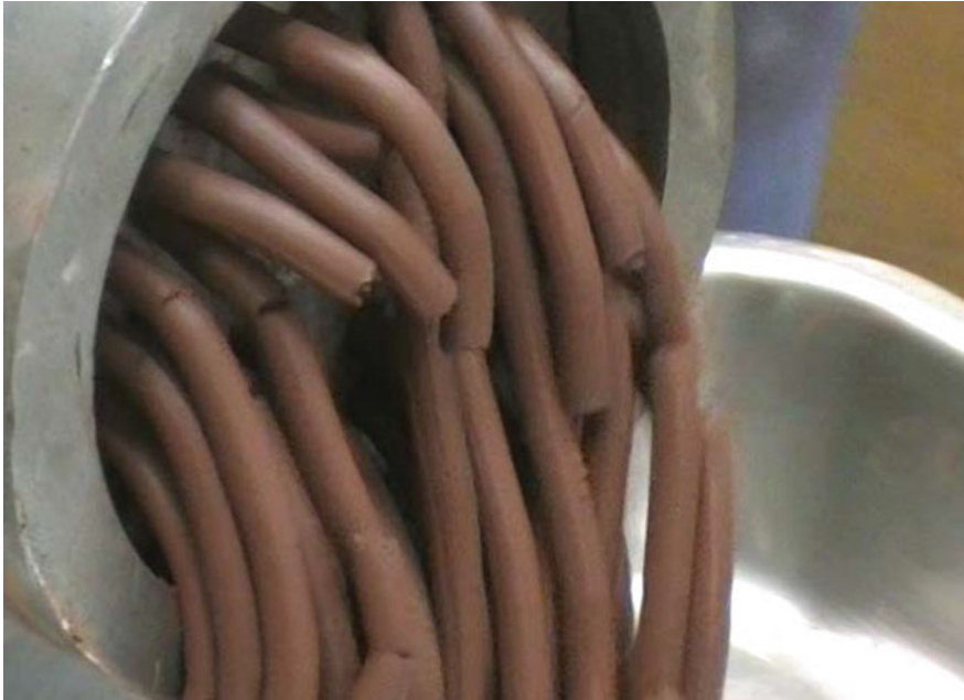
Fig. 6.9 Brex made of red mud with 4% of Portland cement addition
