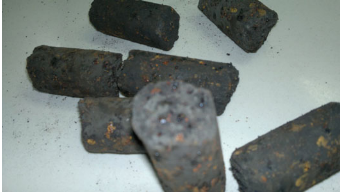
Fig. 5.24 Brex made from DRI fines (at the «Lebedinsky GOK»)
