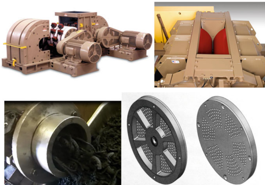
Fig. 2.1 Equipment and tools for materials pulverization (top left—hammer mill; top right—roller crusher; bottom left—shearing through the shearing plate of extruder; bottom right—shearing plate)
