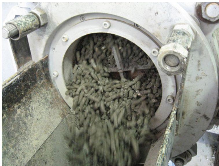
Fig. 6.6 Low-grade Bentonite clay agglomeration by SVE
